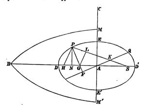
1. Equation to the conic. Draw the arc PN perpendicular to AD and let PN=y, AN=x. Let NP produced cut the small circle described on DD' as diameter in P', let NP' be called the eccentric ordinate and be represented by y'. We then have  $\tan y = \text{constant} = \frac{\tan b}{\tan a}, \qquad \cos a = \cos y' \cos x.$
